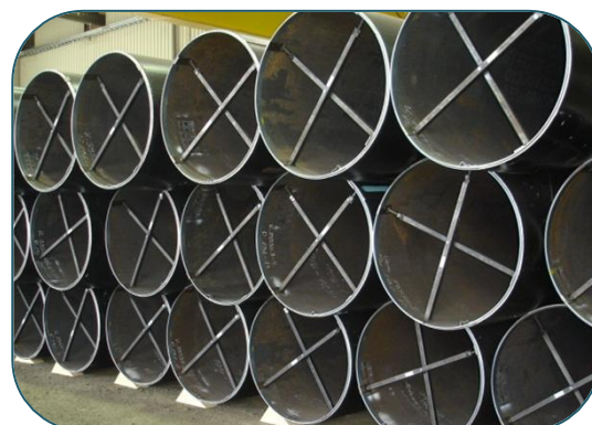
Fig 3: Cross-Bracings in pipes
