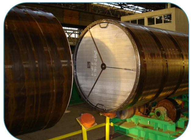
Fig 2: Blasting Plug applied in pipe
