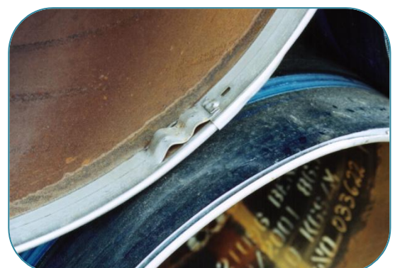
Fig 3: Bevel Protector fitted in pipe-end
